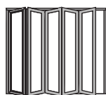
Sistem me palosje 5 kanata Fivefolding door (5 leaves)
